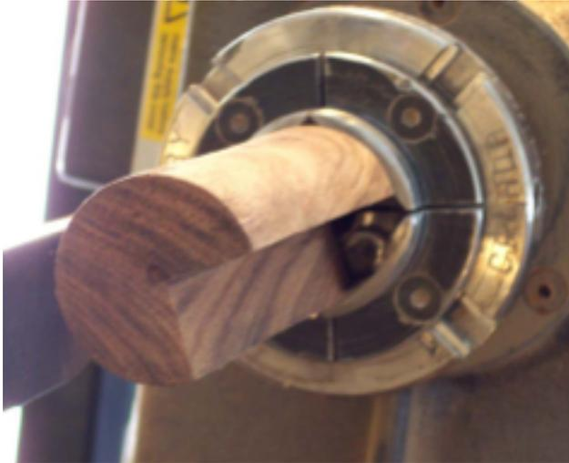
**Here the head is mounted in the chuck and ready to turn. The 1/4 section is left out in the initial turning of the head.**
