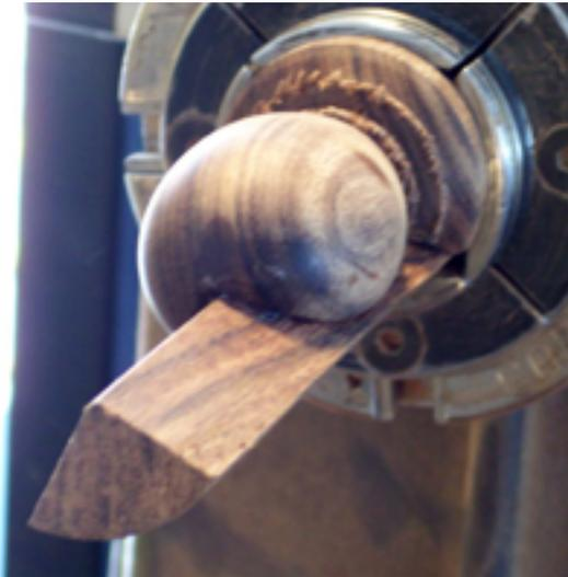
**Here the  $\frac{1}{4}$  section is glued into the head and ready to final turn. You must turn the head down to match with the bill section and turn the bill section to a point at the very end. Do not turn on the center pointed section.**
