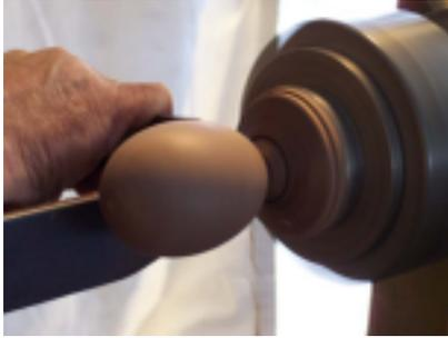
**The body has been turned and is nearly ready to part off. It is easier to turn the body with one end held in a chuck and then you have only one end to hand sand.**
