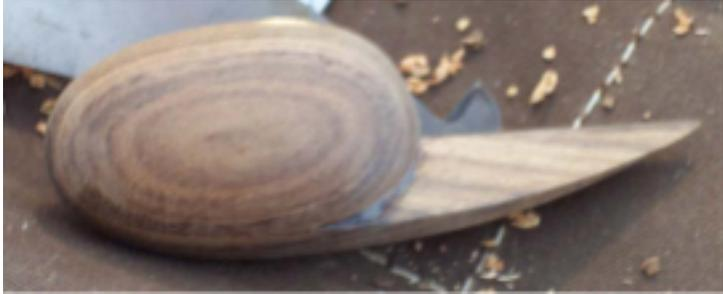
**Here the head has been completely turned. You must hand sand the top of the bill section.**
